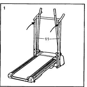
Insert one of the Extension Legs (34) into the treadmill as shown. (Note: It may be helpful to tip the Uprights [11] in the direction shown by the arrow as you insert the Extension Leg.) Make sure that the Base Pad (40) is on the indicated side of the Extension Leg. Attach the Extension Leg with an Extension Leg Screw (53). Make sure to push on the head of the Extension Leg Screw while tightening it.
